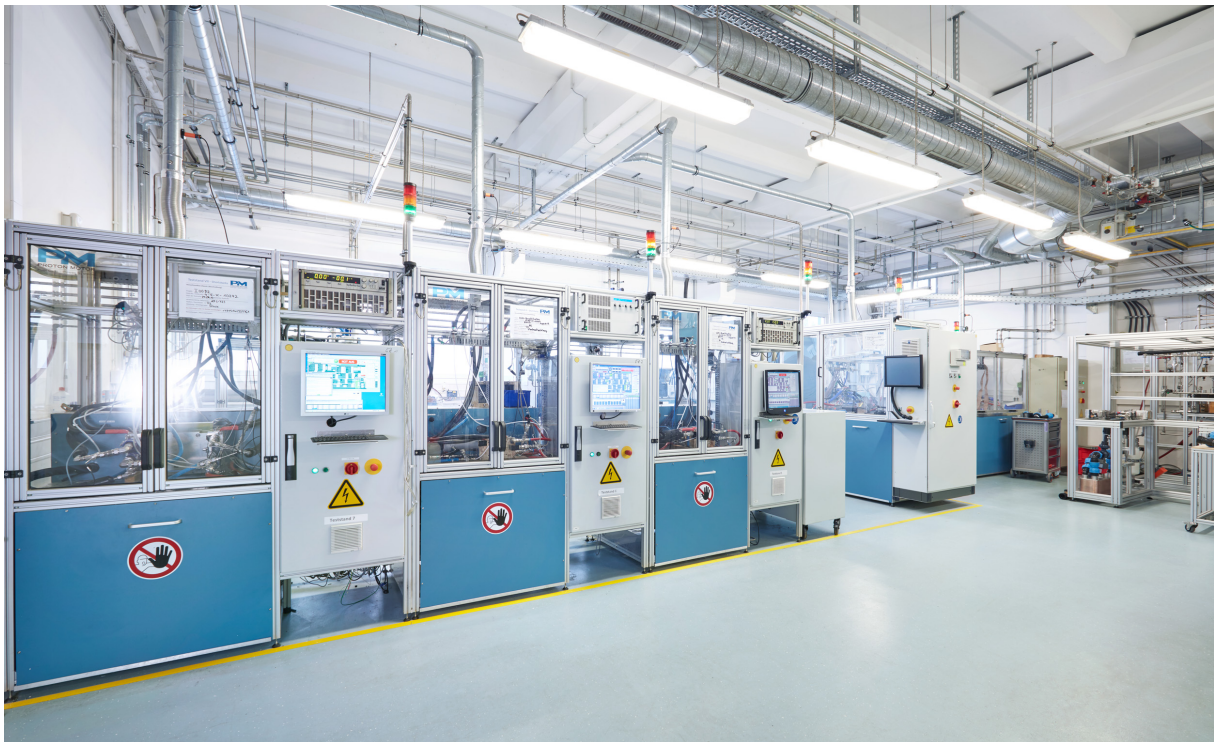
Figure 6 Proton Motor FCS test lab with short stack and full stack test benches
